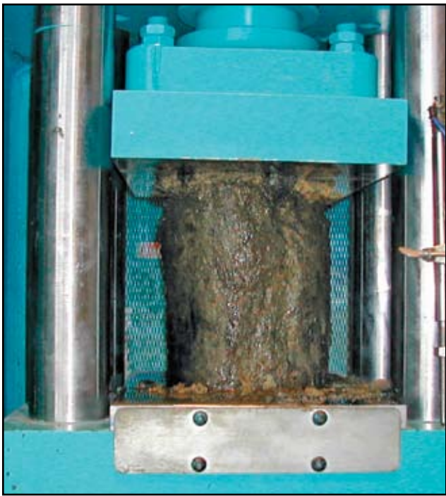
Figure 9: Load test of a full pile cross section.
