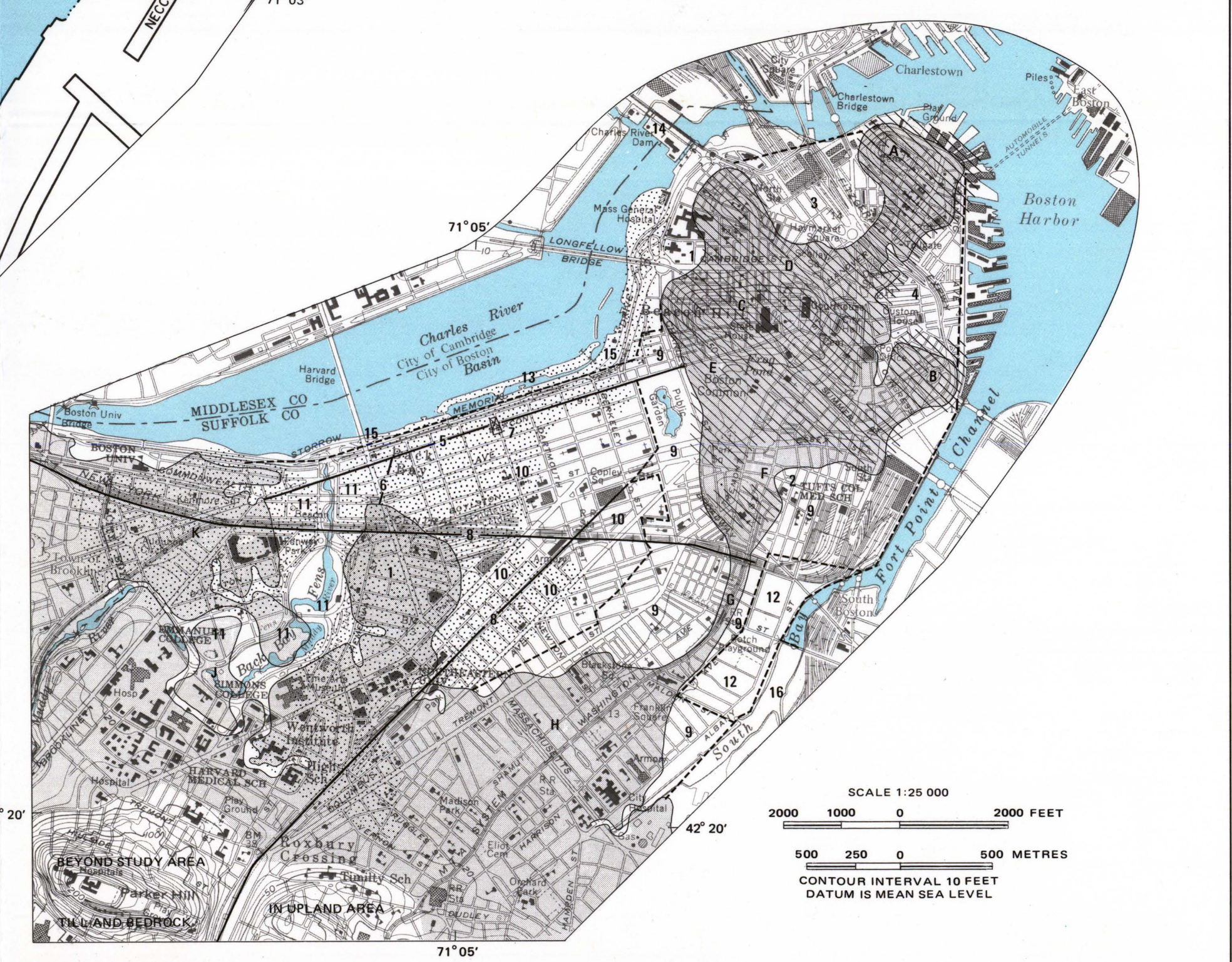
FIGURE 1.—MAP SHOWING ORIGINAL LAND AREA ABOVE MEAN HIGH TIDE, NEAR-SURFACE MATERIALS, AND SEQUENCE OF LANDFILL OPERATIONS.
