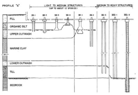
Figure 4. Deep foundations used throughout the decades. (Courtesy of Woodhouse and Barosh, Civil Engineering Practice, *Journal of the Boston Society of Civil Engineers*, 2011-12.)
