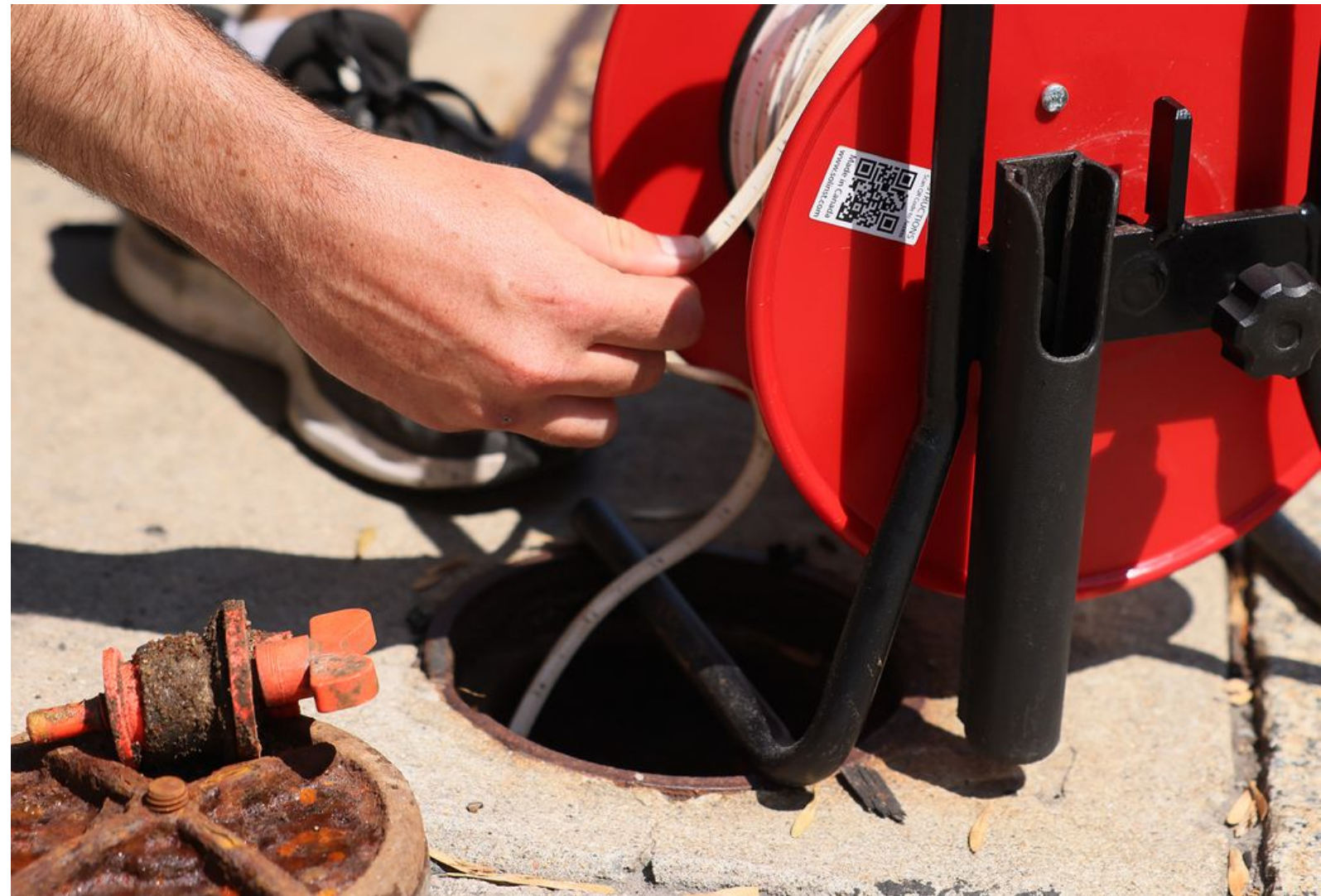
Jake Ryan, a field engineer with the Boston Groundwater Trust, used a water level meter to take a measurement of the groundwater level at a test well in the Fenway. JESSICA RINALDI/GLOBE STAFF
